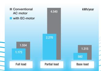
Up to 50 % of the power consumption of a fan can be saved (depending on the operating environment) by the use of EC-motors in place of AC motors.
