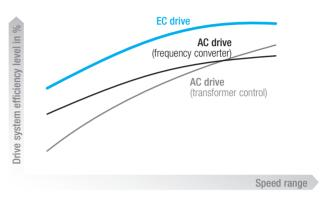
The EC-motor operates without slip losses and thus consumes significantly less power than conventional AC motors.
